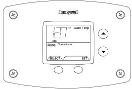
2b. Water Temperature - Upper Sensor (Displays if there is an upper sensor - some models)
